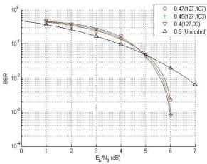
Fig. 5. Performance for GMSK-RS(127;k) code combinations with the same bandwidth as an uncoded system with  $B_bT = 0.5$
