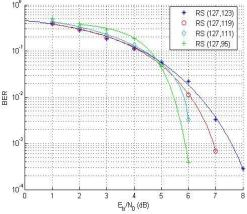
Fig. 9. The BER performance of Reed-Solomon code with increase in Redundancy on codeword 127 having symbol length 7 bits.
