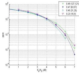
Fig. 8. The BER performance comparison of RS codes for different code rates and different block length but Fix No. of error correction capabilities
