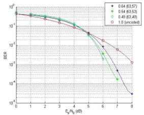
Fig. 6. Performance for GMSK-RS(63;k) code combinations with the same bandwidth as an uncoded system with  $B_bT = 1.0$
