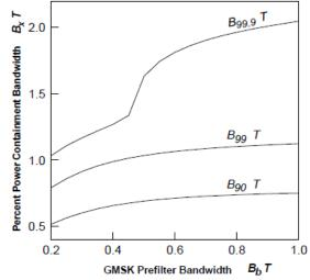
Fig. 2. Percent power containment bandwidths for GMSK
