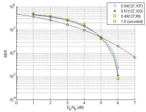
Fig. 7. Performance for GMSK-RS(127:k) code combinations with the same bandwidth as an uncoded system with  $B_bT = 1.0$
