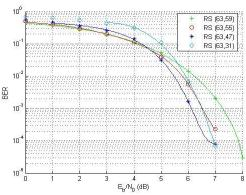
Fig. 10. The BER performance of Reed-Solomon code with increase in Redundancy oncodeword 63 having symbol length 6 bits.
